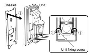
(2) Route the wire through the wire hole in the chassis and secure the chassis in place at the installation location using the detector mounting screws included with the chassis.
